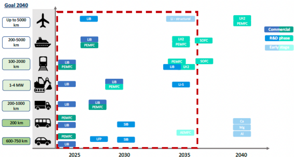
Figure 3: A schematic forecast of the 5-, 10- and 15-year research and implementation perspective. The colours that refer to the different technologies as Commercial, R&D or Early represent the status today, while the placement on the y- and x-axis shows when the first commercial applications are expected, and which type of application will use the technique. Furthest to the left there is also an expected goal for 2040 and the green colour represent how close we are to this goal today.
